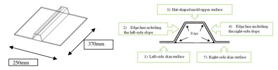
Figure 1: CFRP perform for comparison with experience differences.
